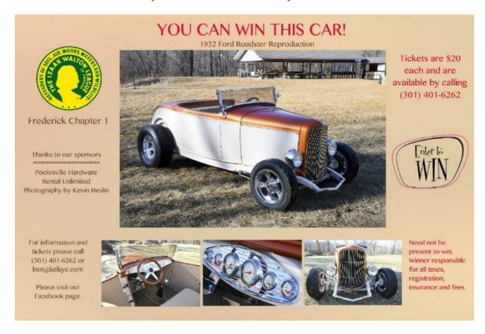
Custom frame, 350ci Chevy Small Block engine, 4 Speed Automatic Transmission, 4 Barrel 650 CFM Classic Holly carburetor, 9-inch Ford Rear Axle, Independent suspension.
